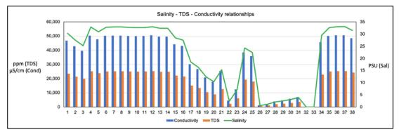
Figure 12: Relationships between salinity, TDS and Conductivity levels.
