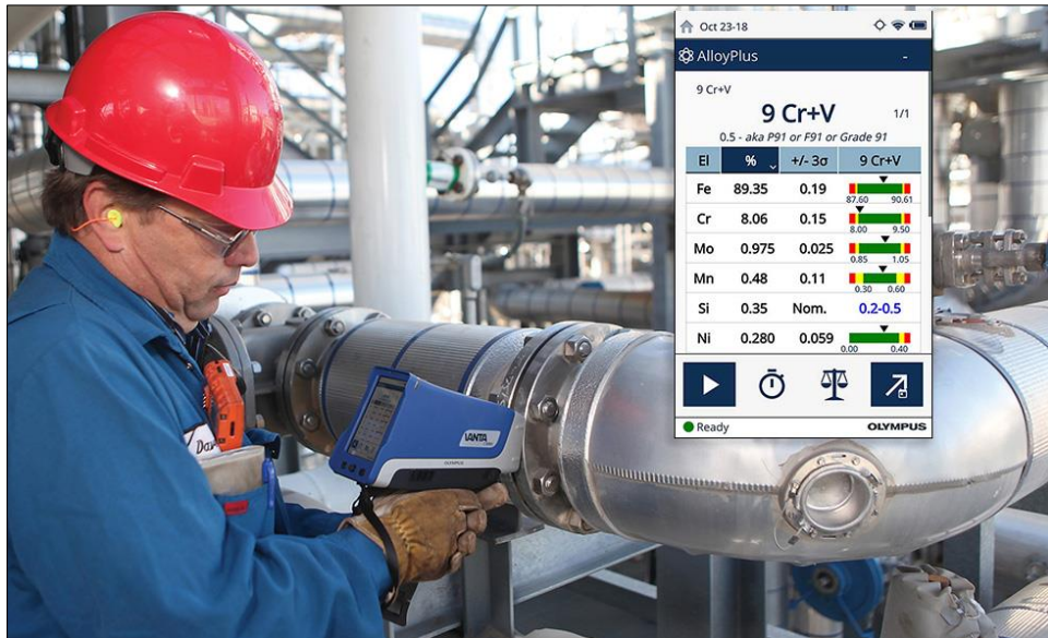
Figure 6. On-site elemental analysis using a handheld XRF analyser to verify pipe alloy composition and identify corrosion risks. Image source: Olympus Corporation.
