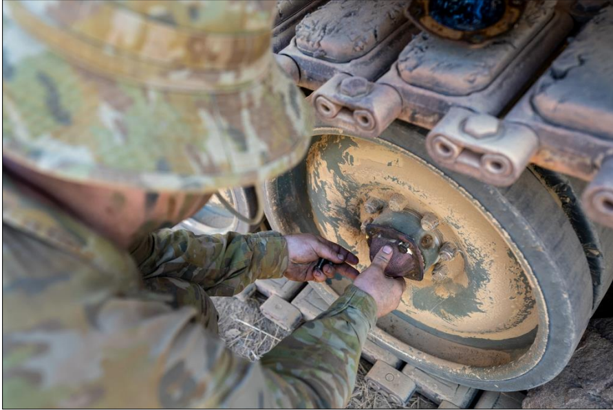
Figure 8. Australian Army installing 3D printed metal wheel bearing cover on M113 Armoured Personnel Vehicle Carrier printed from XSPEE3D printer [54].
