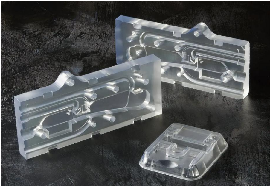
Figure 3. An example of transparent print produced by Vat Photopolymerization [12].
