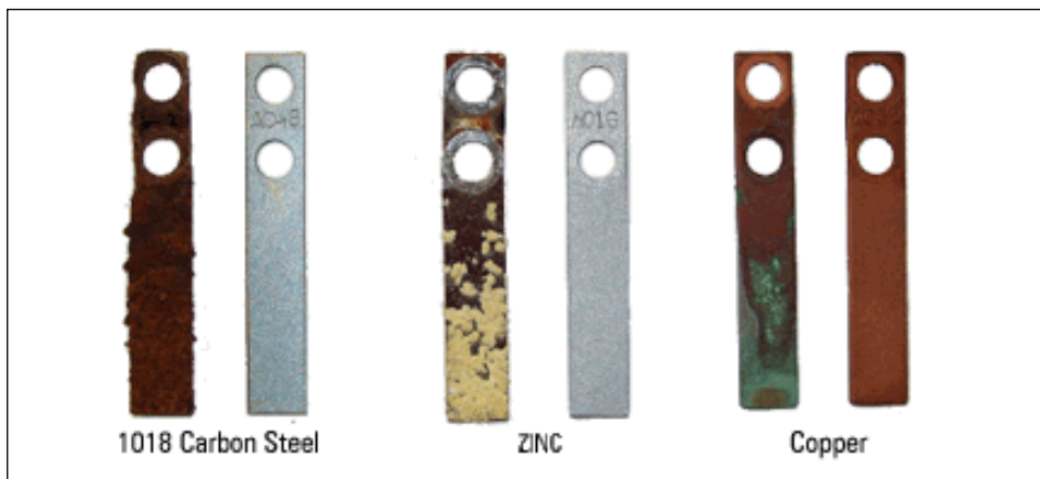
Figure 5. Examples of corrosion coupons made of carbon steel, zinc, and copper before and after exposure. Image source: Caproco Corrosion Prevention Ltd.
