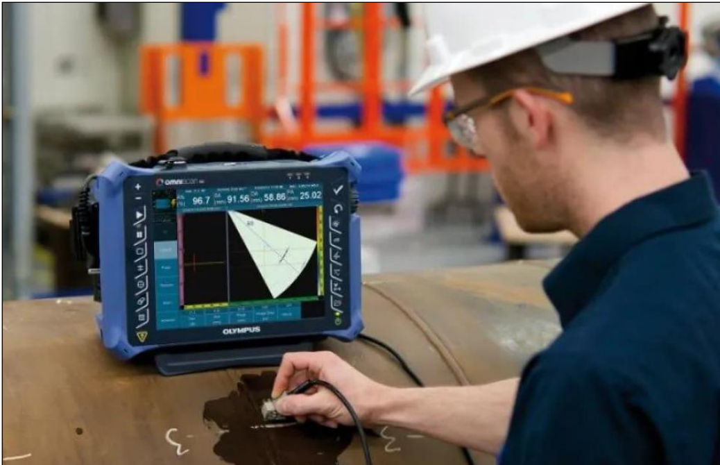
Figure 4. Technician conducting corrosion detection using phased array ultrasonic testing (PAUT). The setup demonstrates real-time imaging for precise flaw detection and thickness measurement. Source: Evident Scientific.
