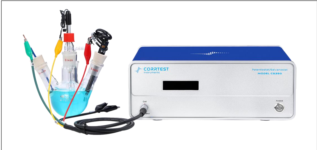
Figure 8. A potentiostat / galvanostat system connected to a three-electrode corrosion test cell for LPR and EIS measurements. The setup includes a working electrode (metal sample), reference electrode, and counter electrode immersed in electrolyte solution. Image source: Corrtest Instruments.
