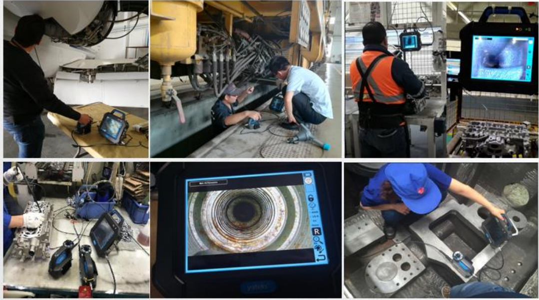
Figure 3. Application of industrial borescopes in various maintenance and inspection scenarios. The handheld devices enable real-time visual inspection of internal structures to detect corrosion, wear, or blockage without disassembly. Image source: Shenzhen Yateks Co. Ltd.
