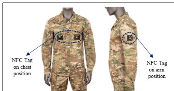
Figure 1: The possible locations of the NFC tag embedded on the soldier's uniform.
