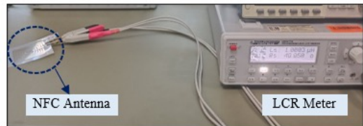
Figure 5: Measurement of antenna inductance and resistance using HM8118 LCR Bridge.
